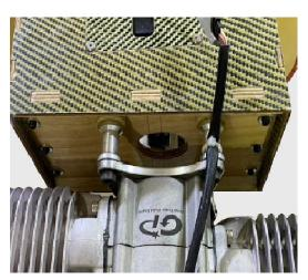
Cut out from paperboard or cardboard as a template for vent hole
