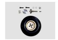
2. Install wheels, secure wheels with gasket and screw. (Apply threadlocker to screws)
